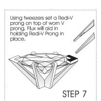
Use a small flame to direct heat on worn prong until solder on bottom of Redi-V Prong flows and adheres Redi-V Prong to worn prong.
