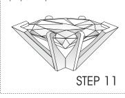
POLISH, CLEAN & INSPECT: Polish ring using your standard prodedure. Clean ring using ultrasonic and steam cleaner. Inspect finished ring.
